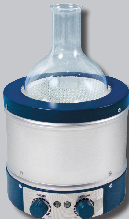
1,000 ml round flask heating mantle
