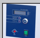
2/4 independent Jog-Shuttle controller
