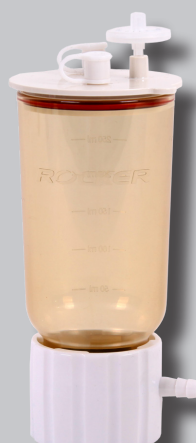
LF 3a - 300ml Ø 47mm, with bottle adaptor
