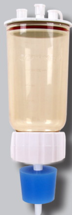
LF 3 - 300ml Ø 47mm, with stopper
